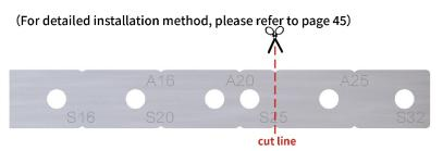
**STED 1** Cut from the guide mark corresponding to the cylinder bore size
